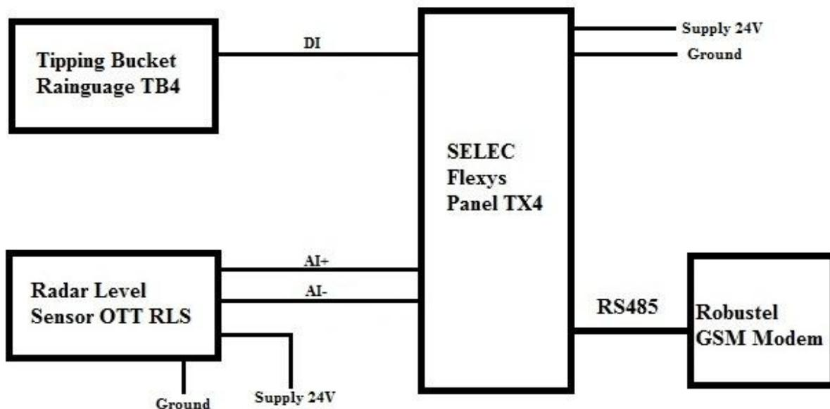
Fig. 1 Connection Diagram of Dam Automation System
