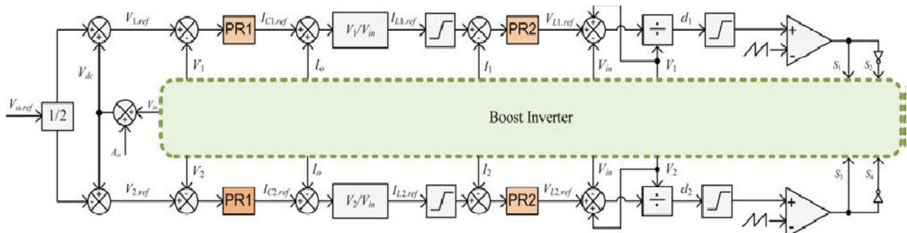
Fig. 2. Boost-inverter control block diagram.
