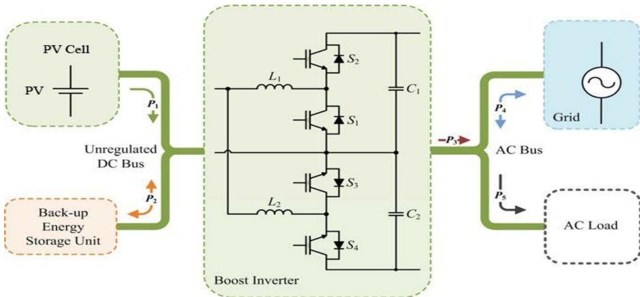
Fig. 1. Block diagram for the proposed grid-connected PV system. The backup unit and the PV power module are connected in the unregulated dc bus and the boost-inverter output is connected to the local load and the grid. (P1: PV output power, P2: backup unit input/output power, P3: inverter output power, P4: power between the inverter and the grid, and P5: power to the ac loads).
