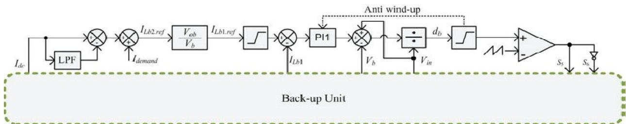
Fig. 3. Backup unit control block diagram.
