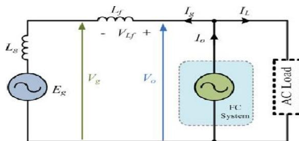
Fig. 4. Equivalent circuit of the grid-connected PV system
