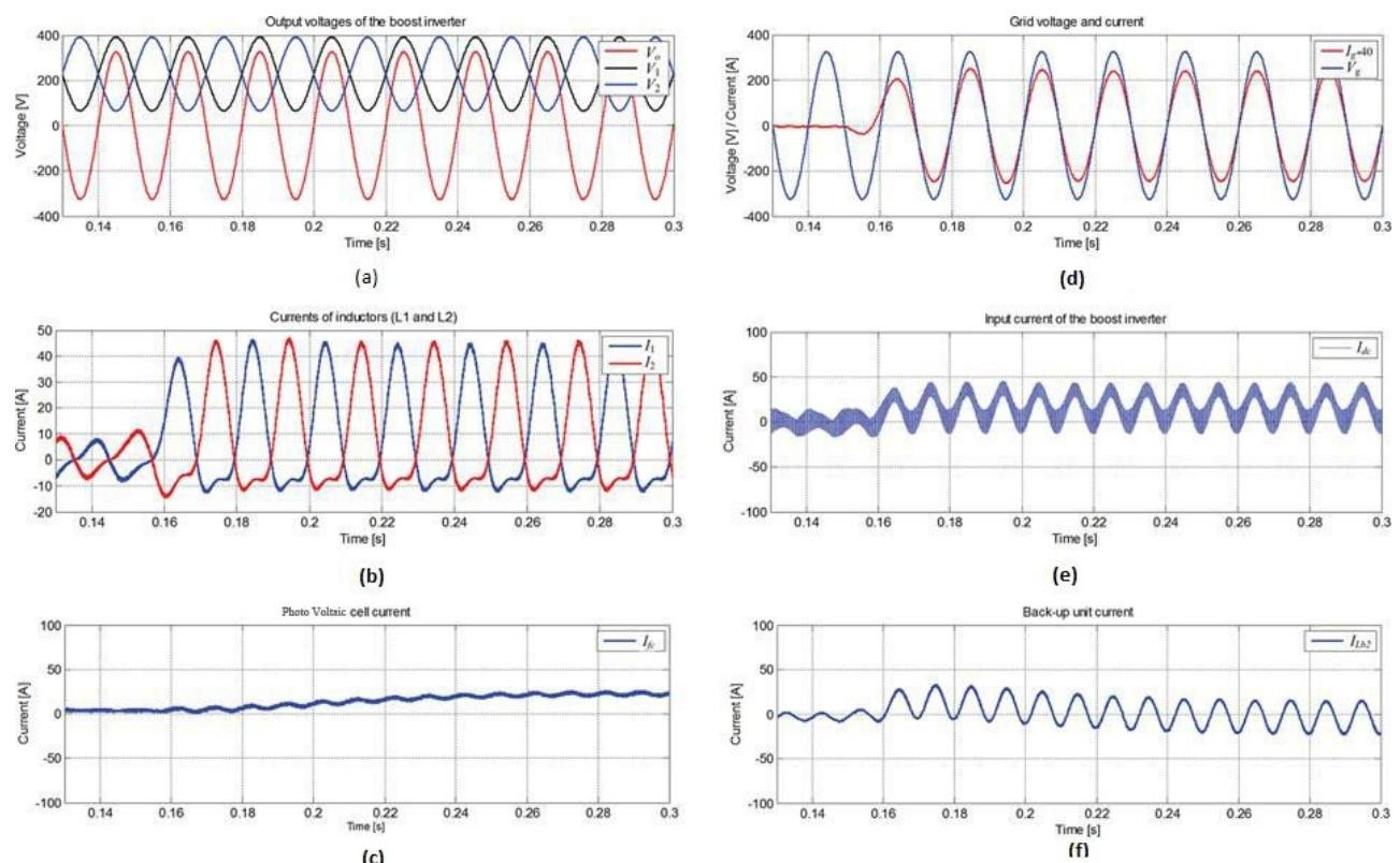
Fig. 6. Simulation results of the proposed PV system. (a) Output voltages of the boost inverter. (b) Current waveforms of  $L_1$  and  $L_2$  . (c) PV output current during transient,  $I_{pv}$  . (d) Grid voltage  $V_g$  and current  $I_g$  with full power feeding to the grid. (e) Input current of the boost inverter,  $I_{dc}$  . (f) Output current of the backup unit,  $I_{LB2}$  .
