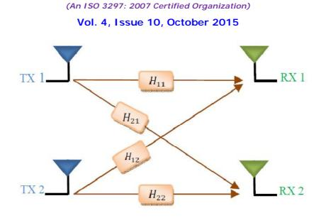
Figure 3. MIMO channel model.
