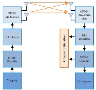
Figure 2. Proposed MIMO-OFDM system model for symmetric channel.
