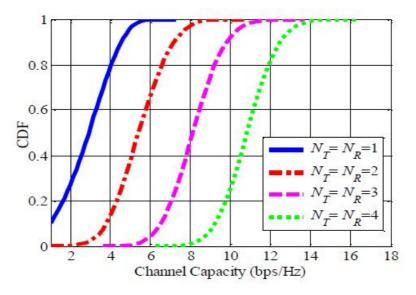
Figure 4. Ergodic MIMO Channel Capacity in Terms of SNR
