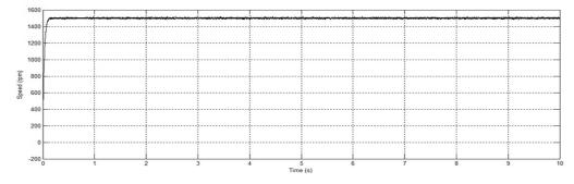
Fig.9 Speed Control of BLDC Motor Drive with Zeta converter
