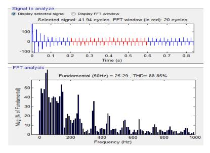
Fig.7 Harmonic Spectra of BLDC Motor Drive without PFC converters
