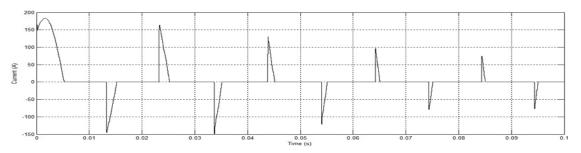
Fig.6 Current waveform at ac mains of BLDCMD without PFC converter
