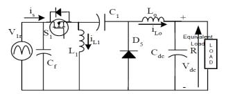
Fig. 1: Circuit of Zeta Converter
