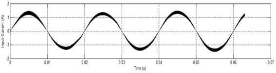
Fig.10 Current waveform at ac mains of Zeta Converter fed BLDC Motor Drive
