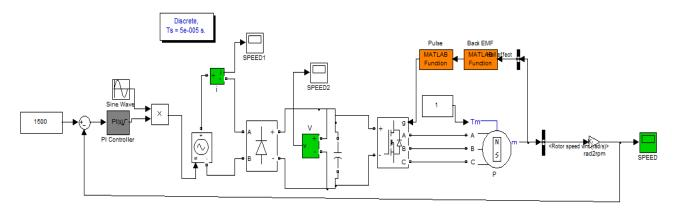
Fig.5 BLDC motor drive without PFC Converter
