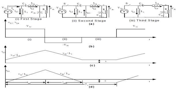
Fig. 2 (a) Three Different Operating Stages (i), (ii) and (iii) of Zeta Converter in DCM of Operation and its (b) Voltage Waveforms (c) and (d) Inductors Current Waveform
