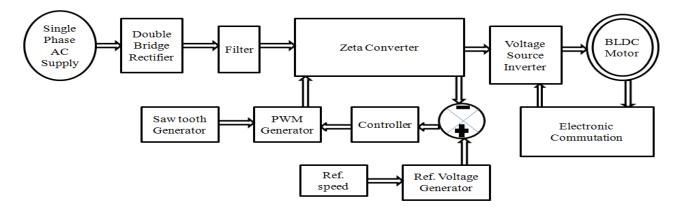
Fig.3 Proposed PFC-based zeta converter fed BLDC motor drive
