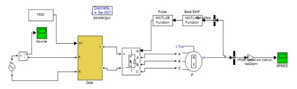
Fig.8 BLDC Motor Drive with Zeta converter for harmonic reduction
