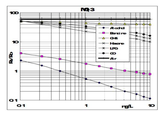
Fig.7 Typical sensitivity characteristics of the MQ-3 for different gases.
