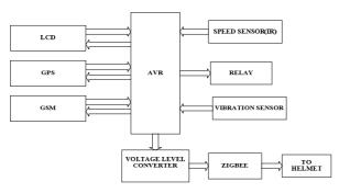
Fig.3 – Block diagram explanation of Bike section
