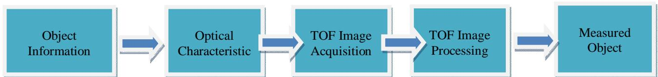
Fig 6. Image Processing blocks for PMD-TOF Camera [7]
