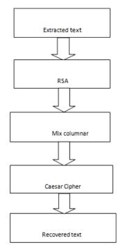
Figure 7: Decoding algorithm
