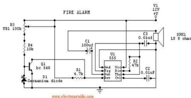
An reverse biased germanium diode is used here as a heat sensor at normal room temperature the reverse resistance of the diode is very high in the order of over 10 kilo ohms so it produce no effects on the transistor Q1 which conducts and keeps the reset pin 4 of ic 555 at its ground level, and so the alarm doesn't get activated.
