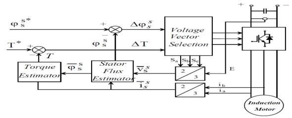
Assuming the voltage drop Rsiss small, the stator flux is driven in the direction of the stator voltage v ss
