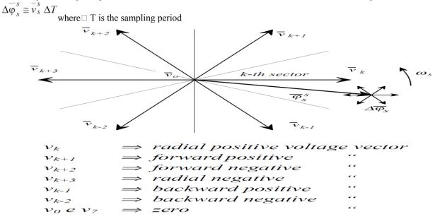
The flux variation is proportional to E,  $\Box$  T and has the same direction of the voltage vector applied ROTOR FLUX AND TORQUE VARIATION
