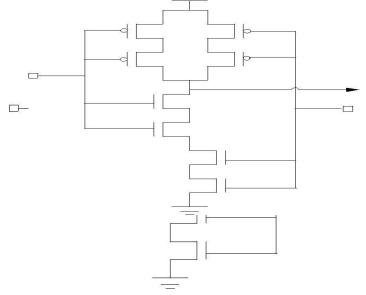
Fig.5.Stack Approach based 2 input NAND gate
