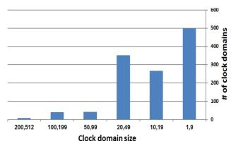
Fig.3.Distribution of the number of FFs sharing a common pre-enabled clock signal of a DSP core
