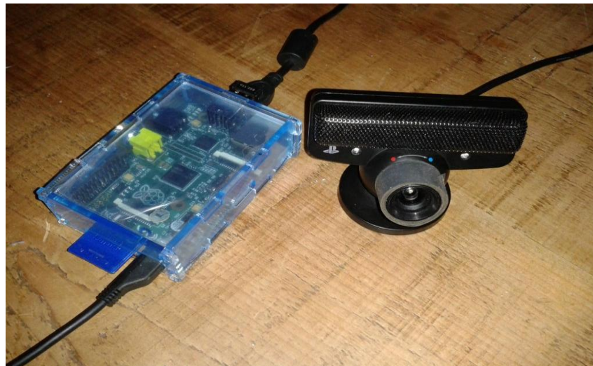
Fig: 3 USB Web Cam Interfaced with the beagle bone Black
