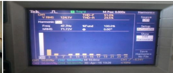
Fig.7 THD measurement on power DSO
