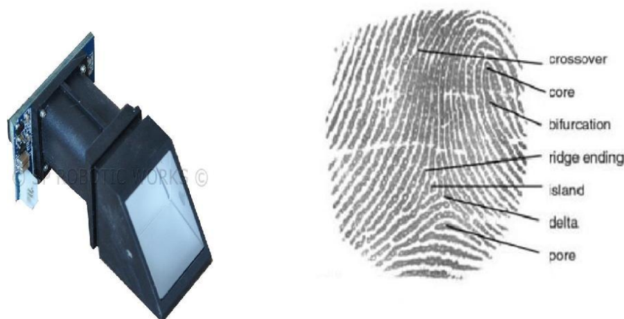
Fig. 4 R305 module and fingerprint recognition with various features
