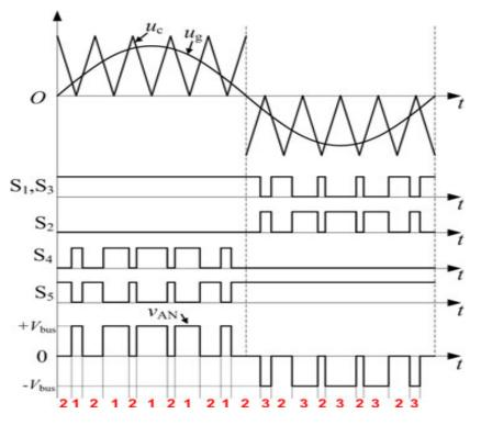
Fig .3 Unipolar Spwm for The Proposed Topology.
