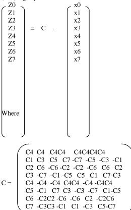
Because the eight-point coefficient structures in MOVING PICTURE EXPERTS GROUP- 1/2/4, STANDARD, and VC standards are the same, the eight-point transform for these standards can use the same mathematic derivation. According to the symmetry property, the 1-D eight point transform in (8) can be divided into even and odd two four-point transforms, Zeand Zo, as listed in (9) and (10), respectively
