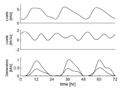
Figure. 5. Microgrid case study II. Powers of loads and generators. Top: sum of active load power. Middle: sum of reactive load power. Bottom: active power of generators.
