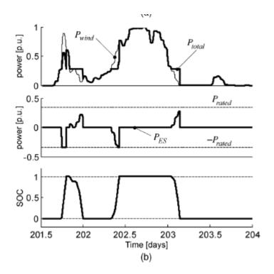
Figure4. Power system of Brekken *et al.* [16]. (a) Wind farm and storage. (b) Optimal solution. Top: wind power and total power. Middle: storage power. 'Bottom: battery SOC.
