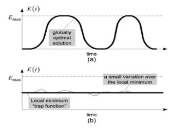
Figure. 3. Global and local solutions in time domain. (a) Global solution. (b) Local solution (bold) with a small variation (thin). The variation is energetically worse than the local solution, due to charge and discharge losses.
