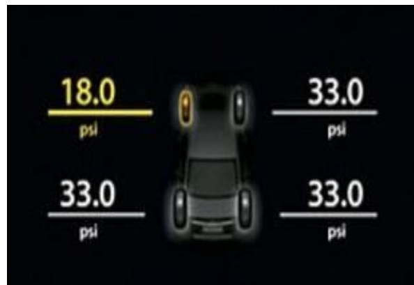
Fig. 9. Tyre pressure display
