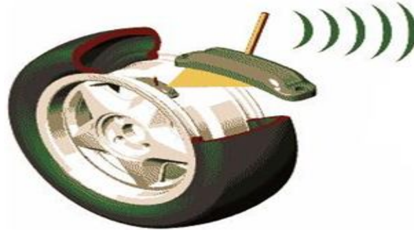
Fig. 4. Transmitter on tyre rim
