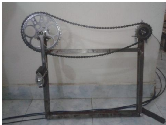
Figure 2: Chain drive along with the stand for the entire setup
