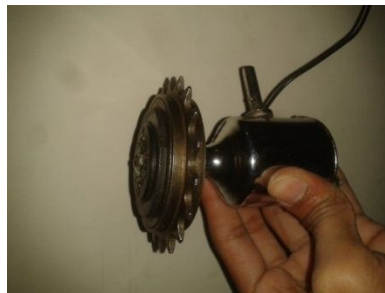
Figure 1: Freewheel attached to the shaft of the dynamo
