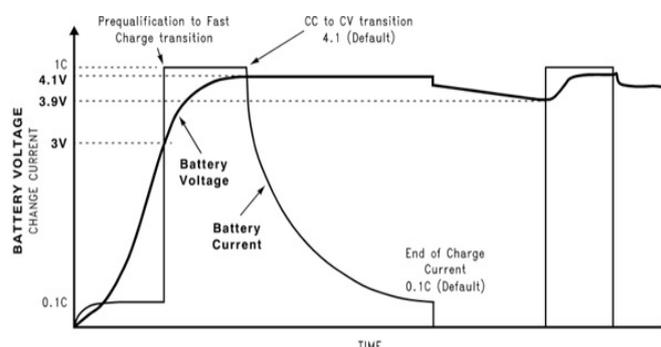
Fig.1. Li-ion battery charging profile
