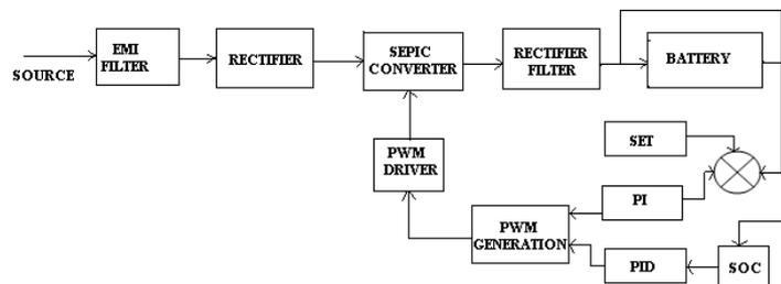
Fig.3. Block diagram of the proposed system
