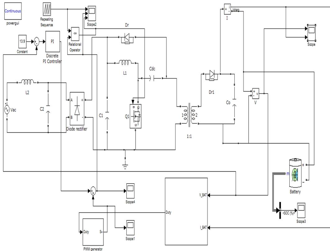
Fig.6.Simulation of the SEPIC based SMPS for battery charger.
