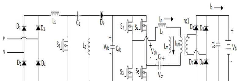
Fig.2. Conventional two stage chargers based on SEPIC PFC and full bridge LLC converter
