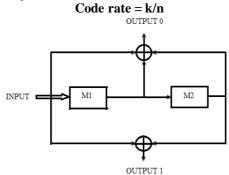
Fig. 2 Convolution Encoder; code rate=1/2, m=2
