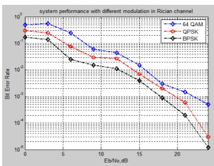
Fig. 8 BER of MIMO-WiMAX system for different modulation with in Rician channel
