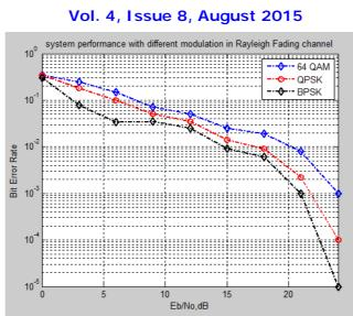
Fig. 7 BER of MIMO-WiMAX system for different modulation with in Rayleigh Fading channel
