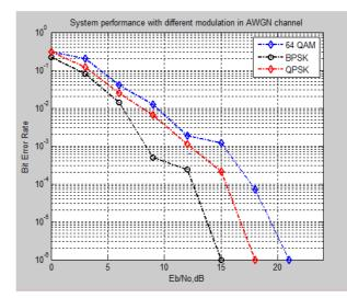
Fig. 6 BER of MIMO-WiMAX system for different modulation in AWGN channel
