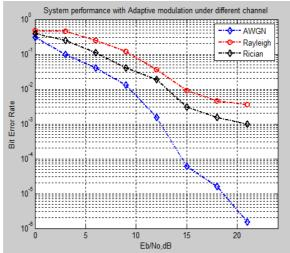
Fig. 9 BER of MIMO-WiMAX with Adaptive modulation under different channel.
