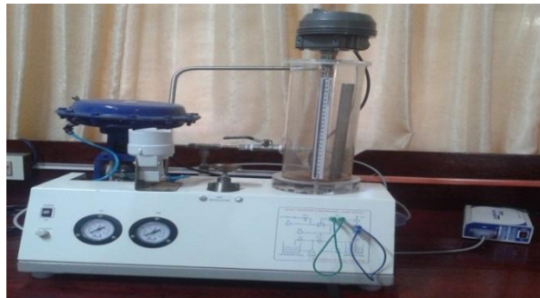
Fig 1: The Liquid Level System under consideration
