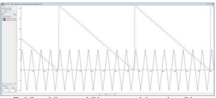
Fig.9 Control Counter and dither counter at below peak condition.
