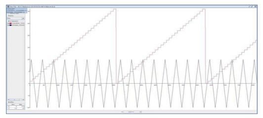
Fig.10 Control Counter and dither counter at above peak condition.
