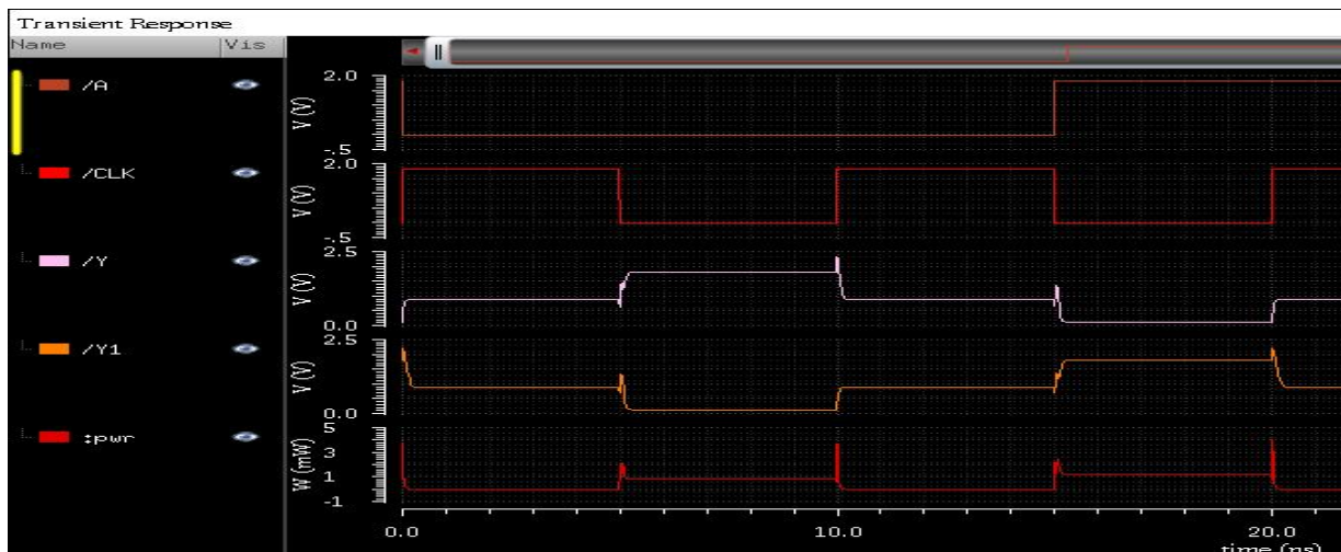
Fig.6 Output waveform for the series of inverters using proposed FTL
