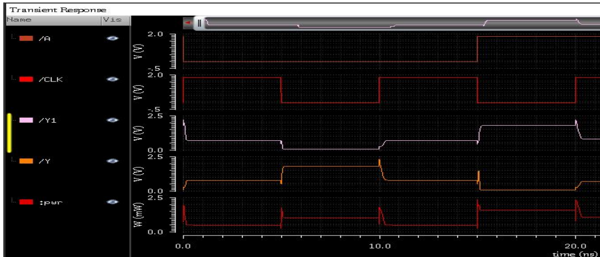
Fig. 5 Output waveform for chain of inverters using high speed FTL
