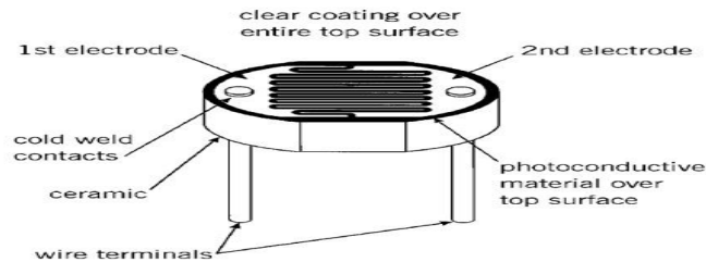
Figure 3 Typical Construction of a Plastic Coated Photocell
