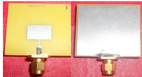
Fig.1 (b) Photographic view of top and bottom MSA
