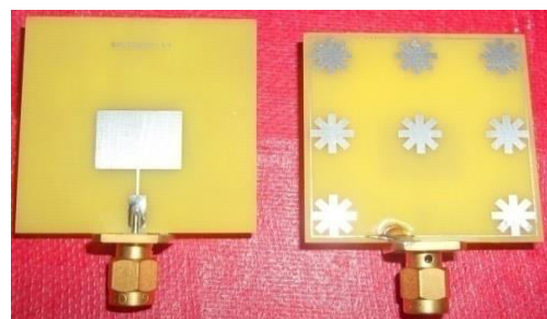
Fig.2 (b) Photographic view of top & bottom of MSAUC-EBG
