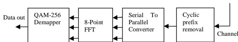
Fig 3: Block diagram of OFDM receiver
