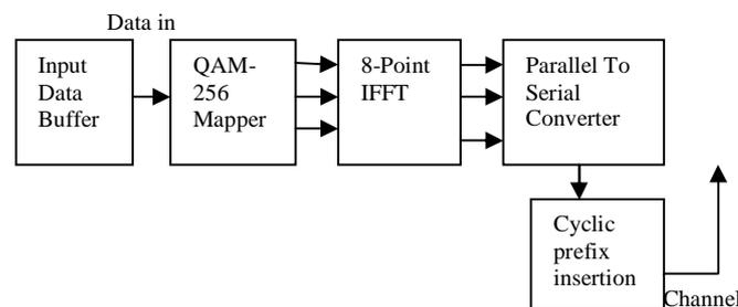
Fig 2: Block diagram of OFDM transmitter
