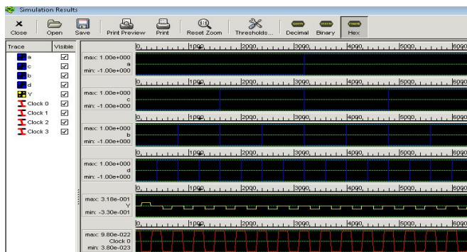
Fig.8.2 Simulation result for four input NOR gate
