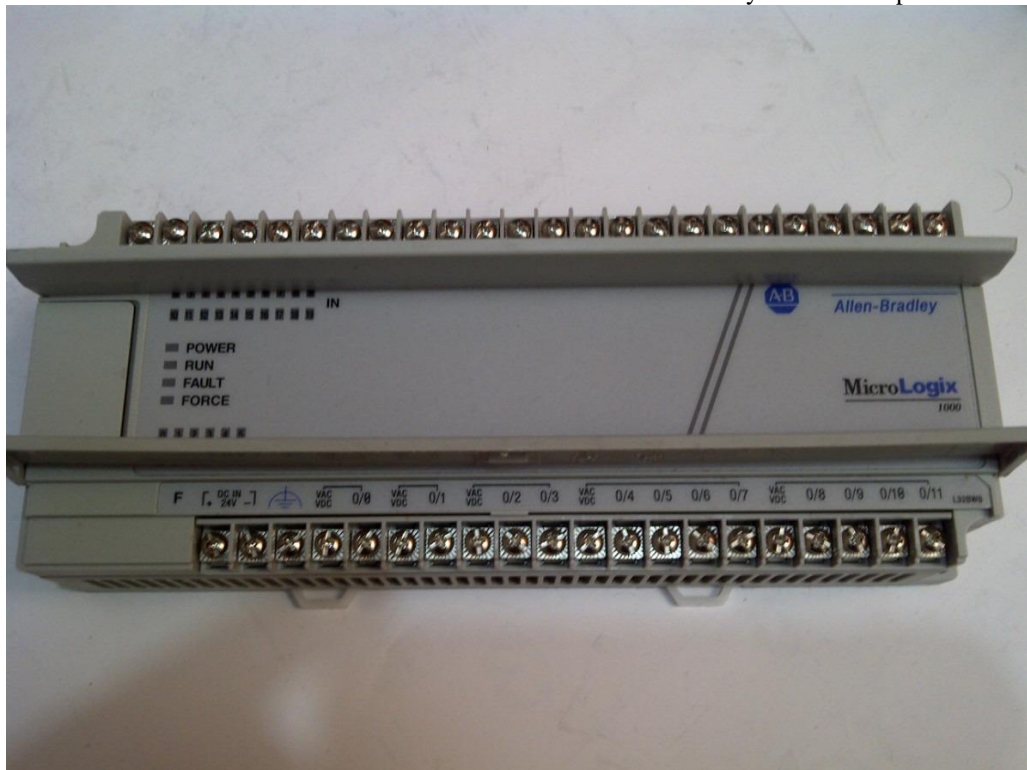
Fig. 4 Allen-Bradley micrologix 1000 PLC [8]
