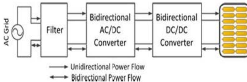
Fig. 2. General unidirectional and bidirectional power flow topology
