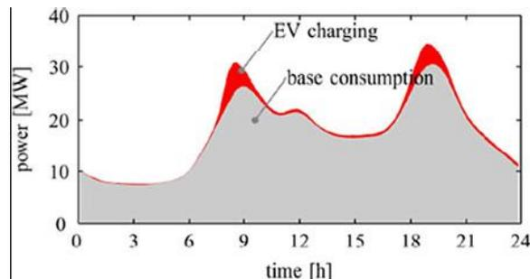
Fig. 3. System base load and total aggregated PEV (2200) charging using uncoordinated direct charging of all the PEVs
