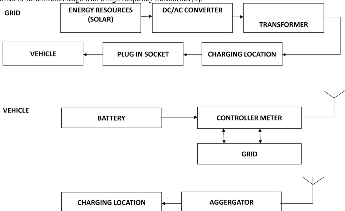
Fig 1:Components and power flow of a V2G system
