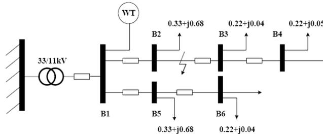
Fig. 7 Test Electricity Distribution Grid (load in MW)
