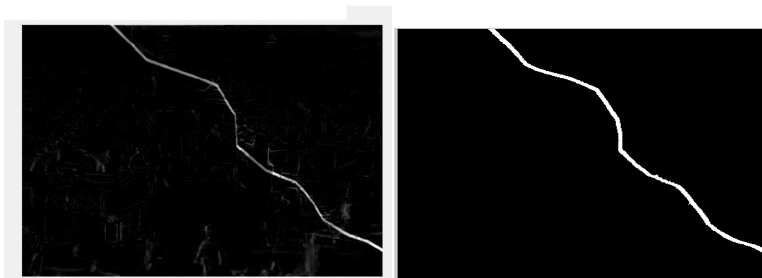
Fig.4 Example of Tear Delineation: (a) Displaced frame difference .(b) Frame after tri map refinement.
