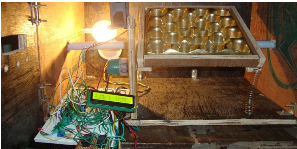
Fig. 5 Inside the Incubator: Lamp, Circulating Fan, Gear motor & Turner assembly, circuit
