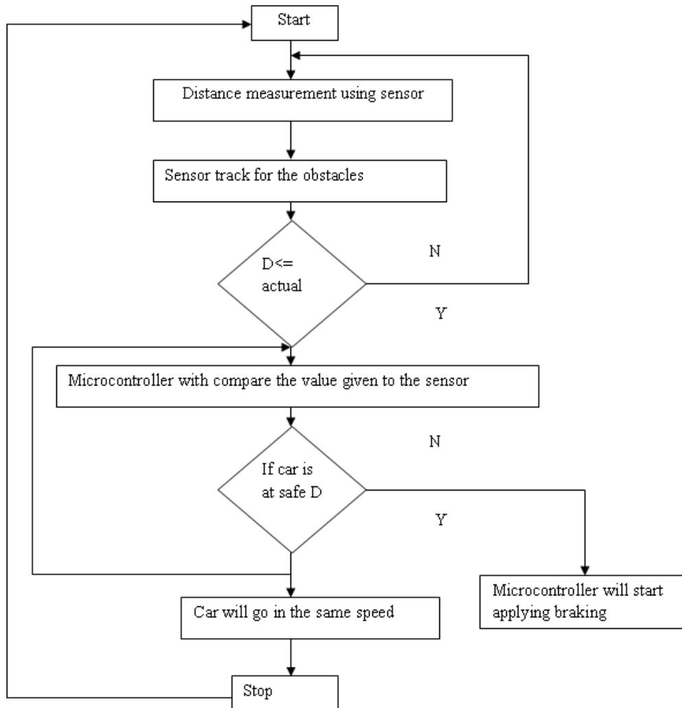
Fig. 5 Flow diagram of detecting obstacle
