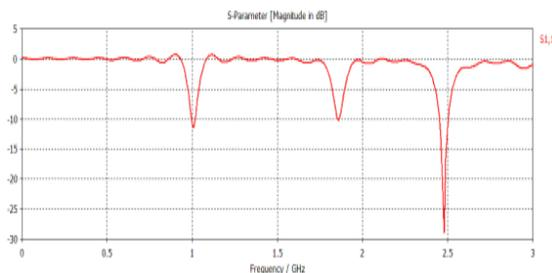
**Fig -7:** Return loss of Sierpinski-PIFA structure
