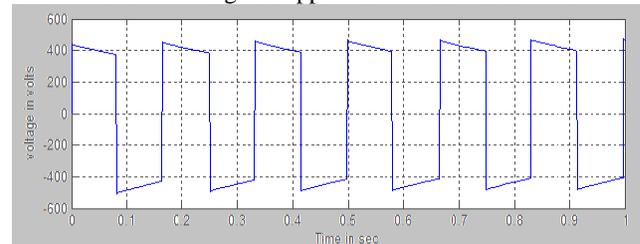
Fig 4 : Pulse Generated using GA approach - operation of STATCOM
