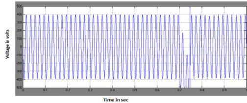
Fig 11: BUS 5 Line Voltage with Fault
