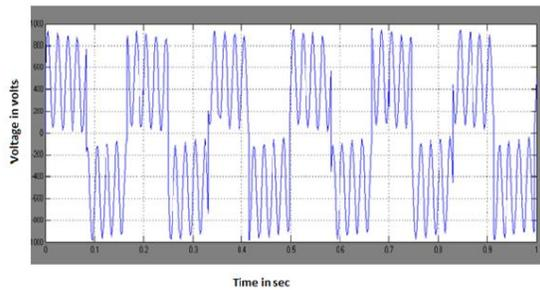
Fig 8: BUS 4 voltage with STATCOM After Fault Occurrence
