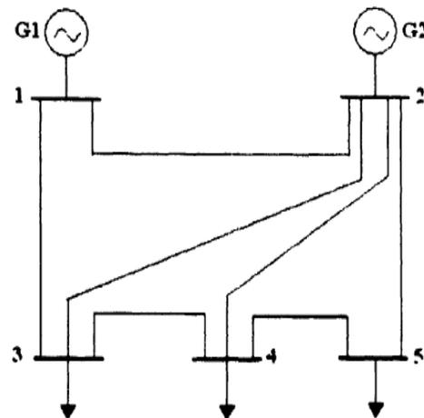
Fig 2: Line Diagram of IEEE Standard 5 BUS System
