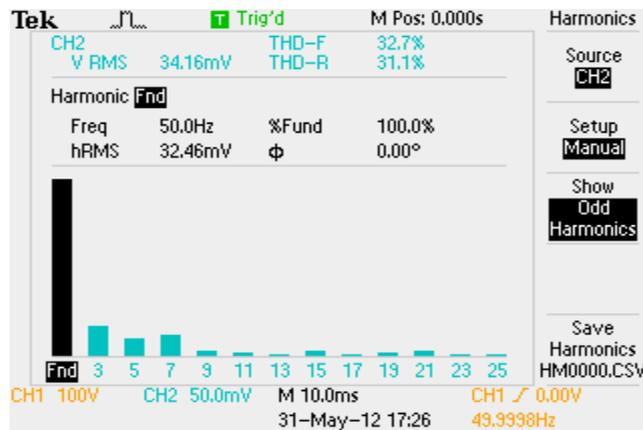
**Fig. 11.** Input current harmonic spectrum of circuit with external PFC
