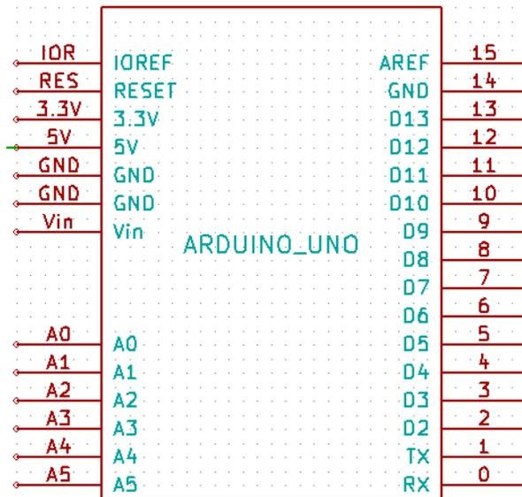
Figure 2: Pin diagram of Arduino Uno board (ATMEGA 328)
