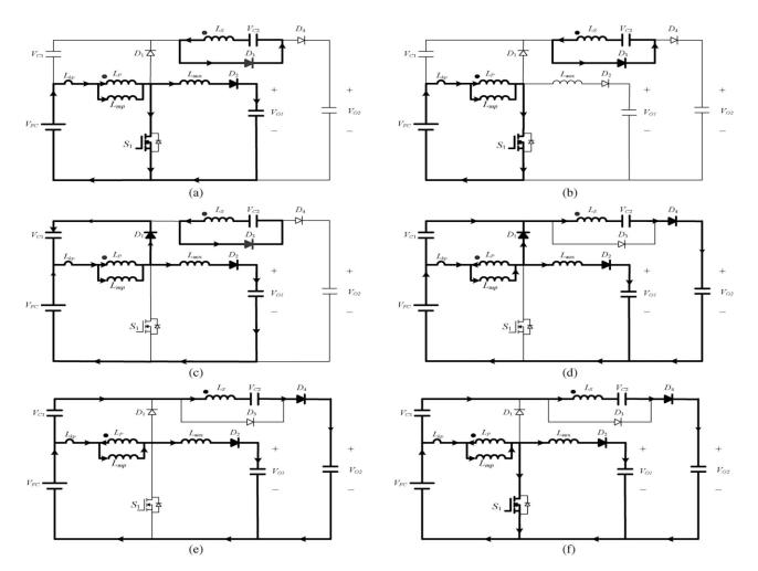
Topological modes: (a) Mode 1 [t0-t1 ]; (b) Mode 2 [t1-t2 ]; (c) Mode 3 [t2-t3 ]; (d) Mode 4 [t3-t4 ]; (e) Mode 5 [t4-t5 ]; (f) Mode 6 [t5-t6 ].
