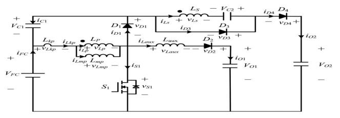
Equivalent circuit of Improved SIMO Converter
