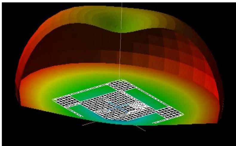
Fig.4: Radiation Pattern of the antenna
