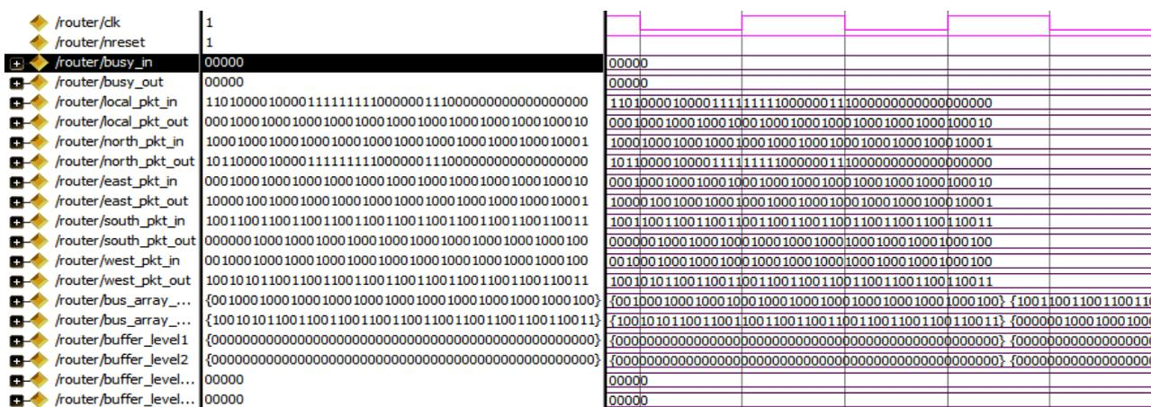
Fig.5 Simulation output with no busy signals
