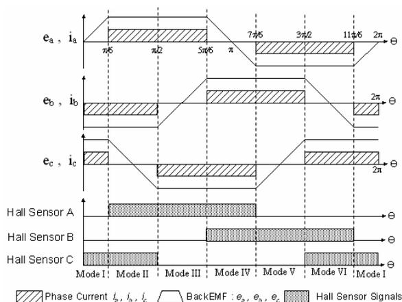
Fig.2. Signal waveforms in the BLDC motor
