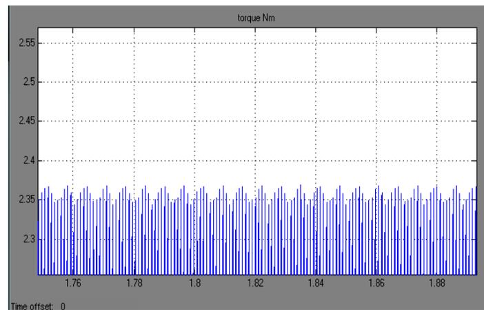
(b) Electromagnetic torque waveform
