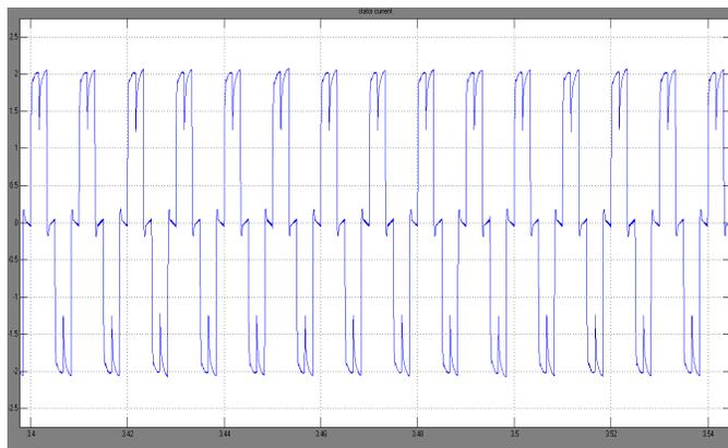
(a) Stator current waveform
