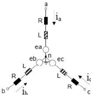
Fig.1. Equivalent circuit of the BLDC motor
