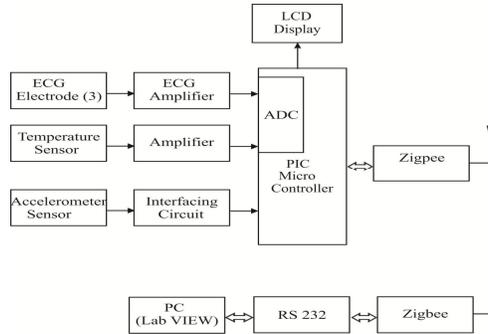
Fig.8 Block diagram for wearable sensors
