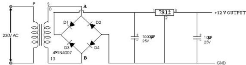
Fig.6 Circuit diagram for power supply
