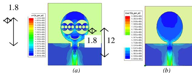
Figure 4: Current Density (a) 3FA Antenna (b) Zeroth Initiator
