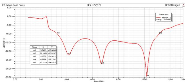
Figure 7: Return loss graph With N notch and ground slit
