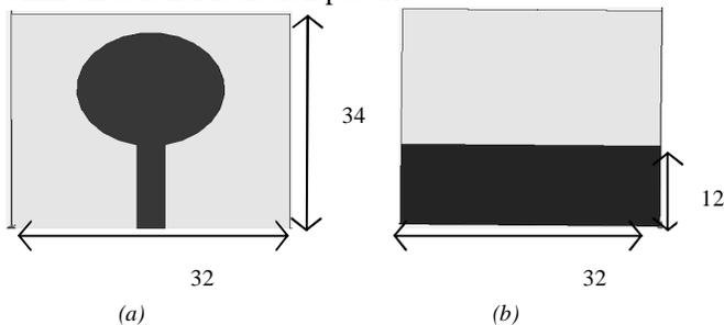
Figure 1: Microstrip antenna (a) Front view (b) Back view (All dimensions are in mm)
