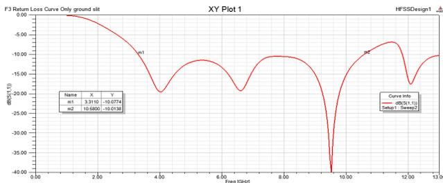
Figure 6: Return Loss graph With Ground Slit
