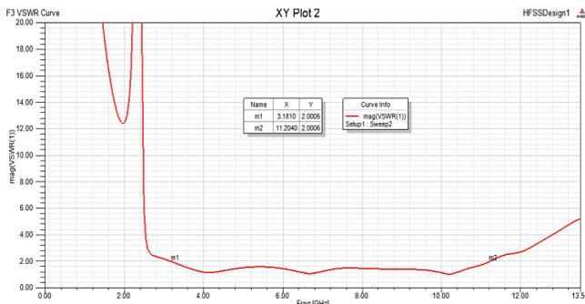
Figure 12: VSWR curve for 3FA Antenna
