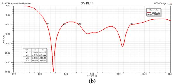
Figure 5: Return loss graph (a) First Iteration (b) Second Iteration
