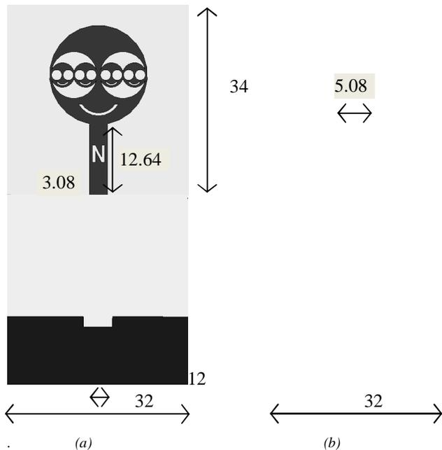
Figure 3: 3FA Antenna (a) Front view (b) Back view (All dimensions are in mm)
