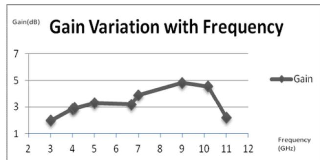
Figure 13: Variation of Gain with frequency
