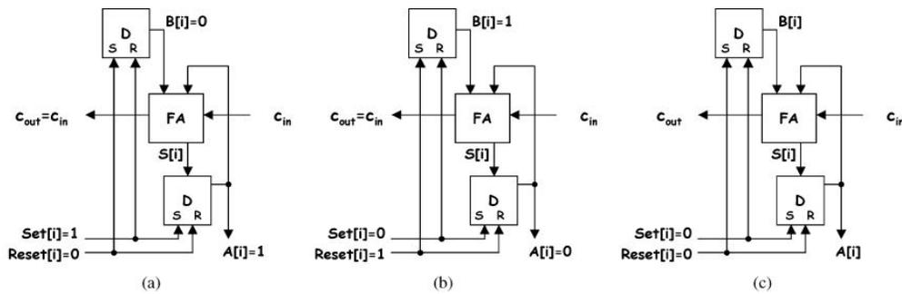
FIG.1: Configurations of the Accumulator Cell.
