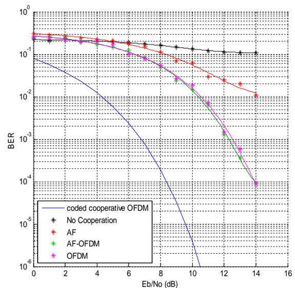
Fig.3.BER comparison between AF relaying and coded Cooperative OFDM systems
