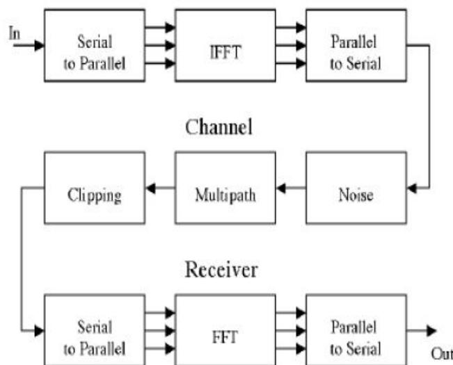
Fig.1.OFDM System Model
