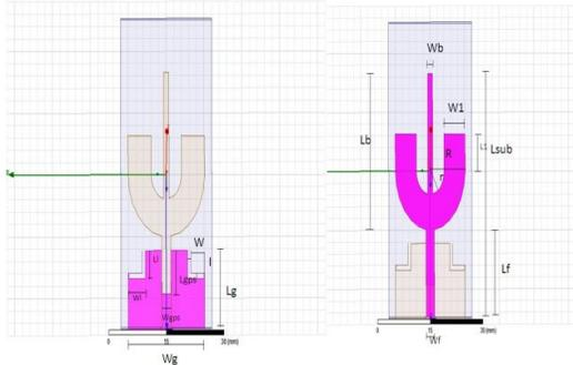
Fig 1: GEOMETRY OF PROPOSED ANTENNA
