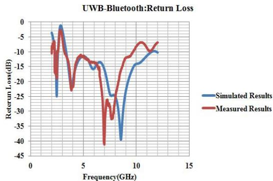
Fig 10: UWB and Bluetooth Return loss
