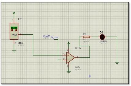
Fig 6. Simulation at 64 Degree Celsius – LED not glowing
