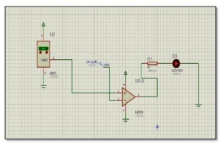
Fig 7. Simulation at 66 Degree Celsius - LED glows
