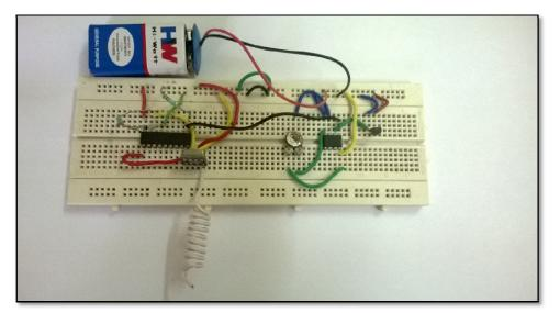
Fig 9. RF Module - Transmitter
