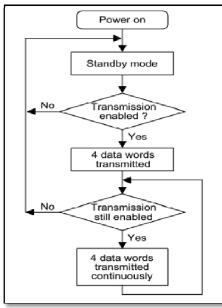
Fig 3. Flow Chart of Encoder IC
