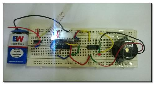
Fig 10. RF Module – Receiver
