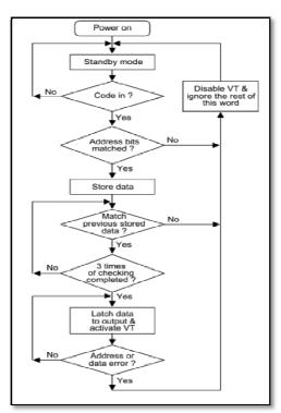
Fig 4. Flow Chart of Decoder IC
