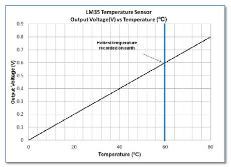
Fig 8. Temperature vs Voltage Variations for LM 35
