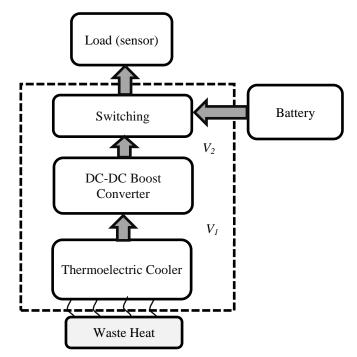
Fig. 2 Block diagram of the designed thermoelectric power source
