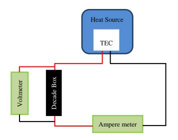
Fig. 4 Experiment circuit of TEC characterization
