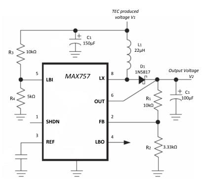
Fig. 3 Schematic circuit of the designed DC-DC Boost Converter
