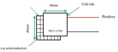
Fig. 1 Thermoelectric cooler structure
