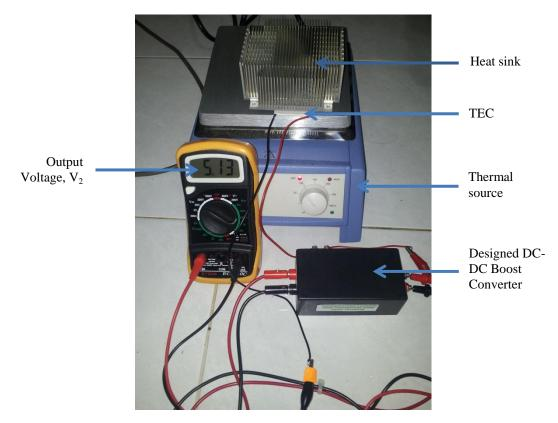
Fig. 7 Experiment Setup
