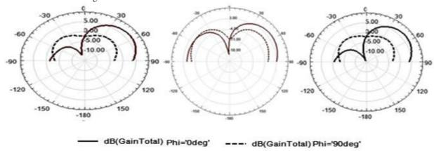
Fig [4] Radiation pattern Curves a) EBG at the end of Ground b) EBG outside the Ground c) EBG on the Ground.
