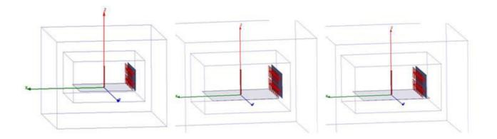
Fig [2] Antenna Design a) EBG at the end of Ground b) EBG outside the Ground c) EBG on the Ground.
