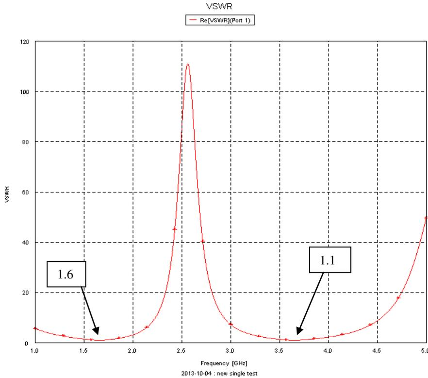
Fig. 3(b) VSWR for proposed dual band antenna
