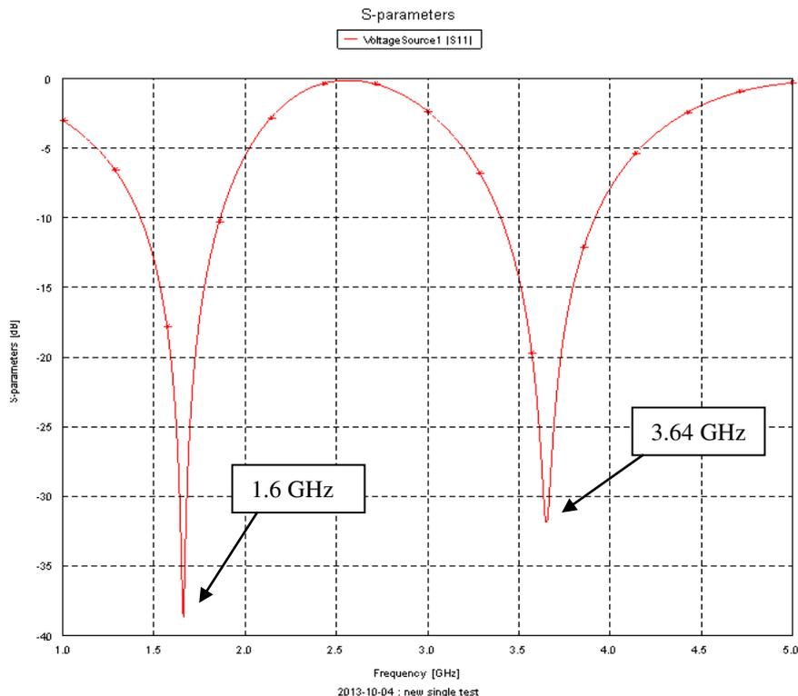
Fig. 3(a) Simulated results of  $S_{11}$  parameter
