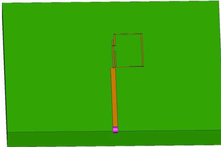
Fig. 1 (a) The proposed dual-band resonating structure microstrip antenna
