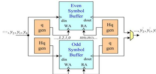
Fig1: Block diagram of typical symbol deinterleaver design
