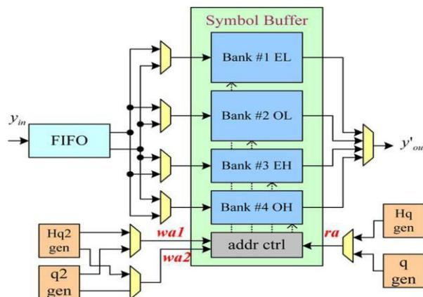
Fig 3. Overall architecture of the proposed symbol-deinterleaver design
