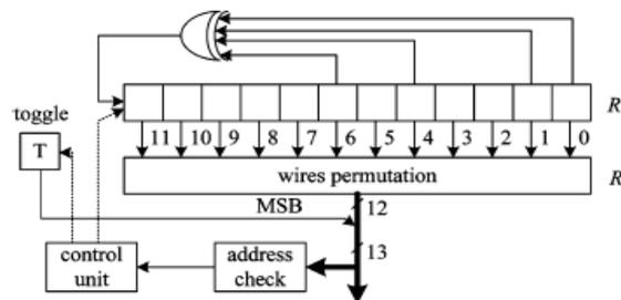
Fig 2. Symbol interleaver address-generation scheme for the 8k mode
