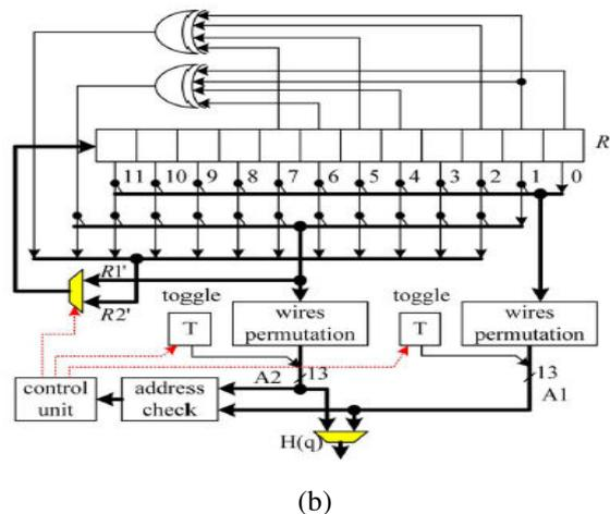
Fig. 5. Proposed design of the permutation function generator: (a) the proposed lookahead algorithm and (b) the detailed circuit diagram for 8k mode.
